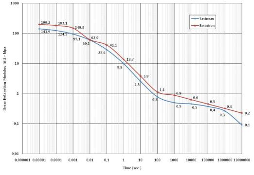
Fig. 4 - PVB shear relaxation modula G(t) vs. time
