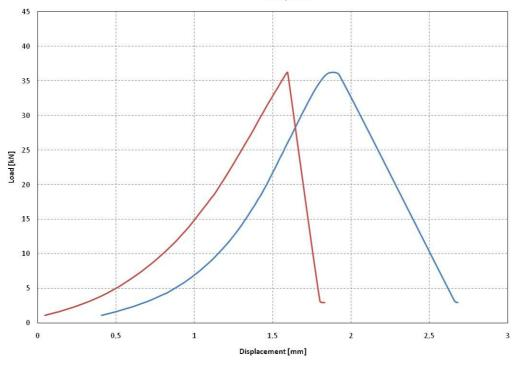
Fig. 3 - Load vs. Displacement for R1-5A specimen
