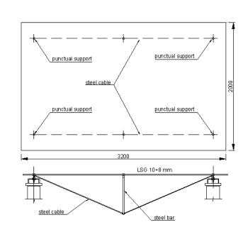
The two specimens, respectively thermally and chemically tempered, were submitted to three different stages of laboratory tests essentially in order to evidence how the Poly-Vinyl-Butyral (PVB) was able to transfer shear stress between the multiple layers under the action of thermo-mechanical load histories.
