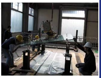
Figure 8 Load application with cylindrical steel weights
