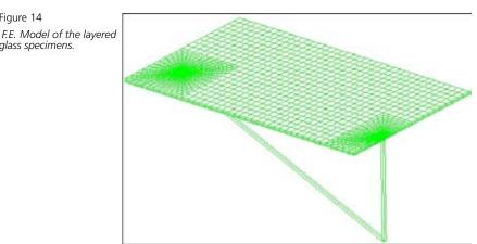
the thickness of the glass elements that cannot be performed with other simplified models. Figure 14 reproduces the F.E. meshing adopted for the two specimens where solid elements and interface elements can be distinguished. The number of mesh knots in each layered plate resulted about 35000 and the number of elements round 7500.
