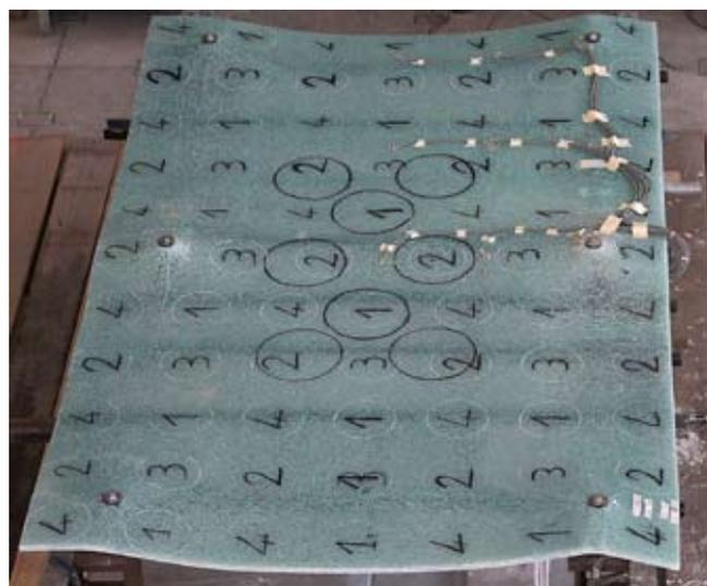
not compromised the residual bearing capacity of the structure thanks to the action of mutual connection performed by PVB. Despite the premature damage we still submitted it to the same final load sequence applied to the specimen TT with the aim to test the post cracking structural behaviour of the plate [Kott, A., Vogel, T., 2003].
