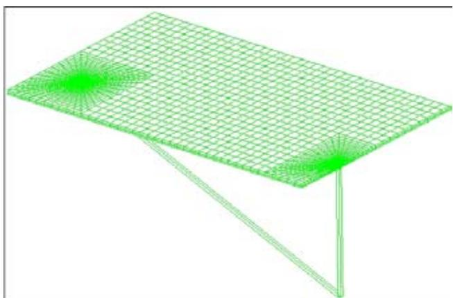
the thickness of the glass elements that cannot be performed with other simplified models. Figure 14 reproduces the F.E. meshing adopted for the two specimens where solid elements and interface elements can be distinguished.
