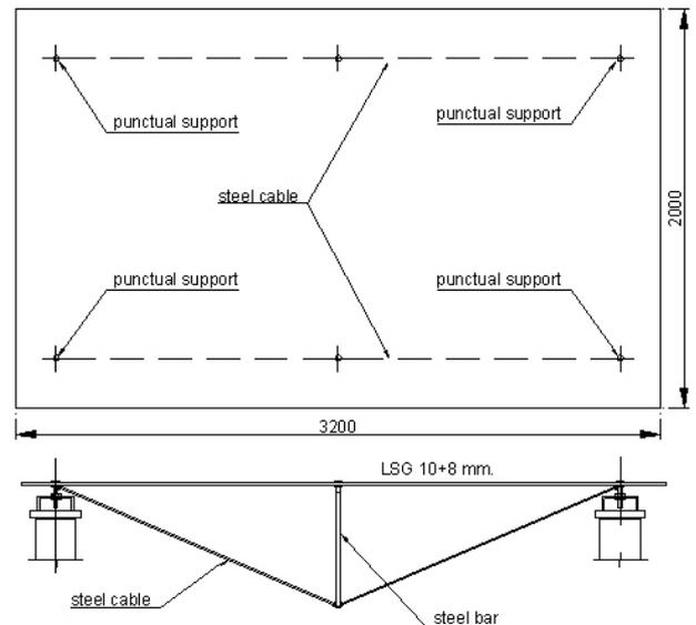
In order to evaluate in advance the critical ultimate bearing ability of the standard element, some modules were tested at the University of Innsbruck under uniform loading [ Böck, et Al.; 1998] actuated by the direct application of bags filled with sand on glass panels put in horizontal position and supported in the same way as those to be used in the construction.
